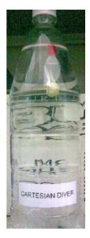
SOY SAUCE 'FISH' Free Cartesian diver. It's best to balance the buoyancy in an open container like a beaker first.
