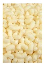
STARCH SOLUTION – a few starch "beans" added to hot water can be used as a starch solution if an accurate concentration is not required.
